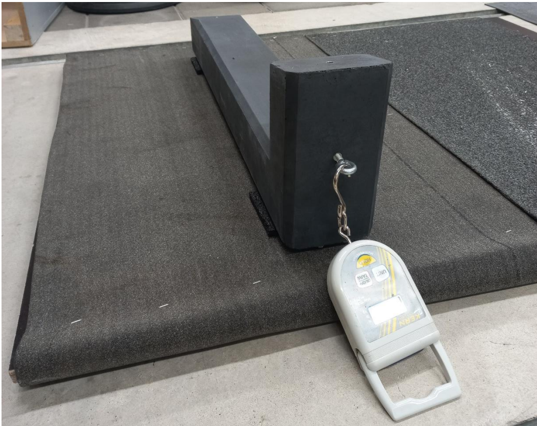
f 1.1 Measurement setup of bituminous roofing
